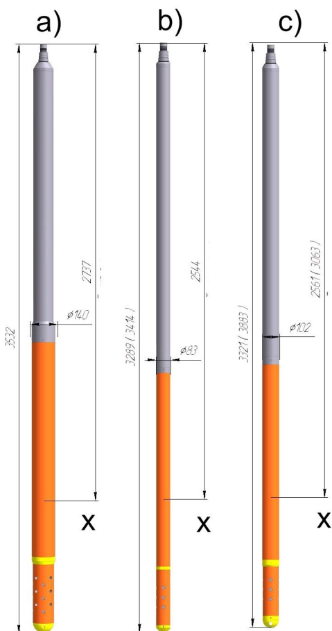
Fig. 1. Earth's field NMR tools family: a) – NL8 – OD 140mm; b) – MRL9 – OD 100mm; c) NL9 – OD 80mm; x – recording point
